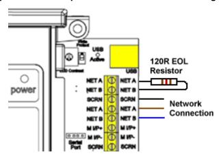
On the repeater a  $120\Omega$  End of Line (EOL) resistor must also be fitted across A and B but only on the last repeater on the network.
