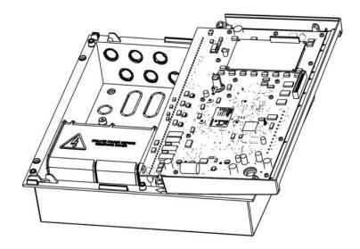
6. Secure the expansion card PCB to the unit's base using the 4 off M3 x 6 screws supplied. Please note the orientation of the expansion card PCB.
