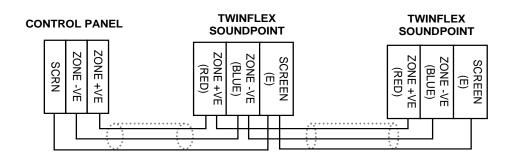
Twinflex Soundpoints can be mixed on the same zone as other types of Twinflex device (eg. Twinflex Multipoint Detectors). The above diagram shows how to make the zone positive, zone negative and screen connections between the control panel and Twinflex Soundpoints. Refer to the instruction leaflets supplied with other Twinflex devices for their equivalent wiring/terminal labelling details.
