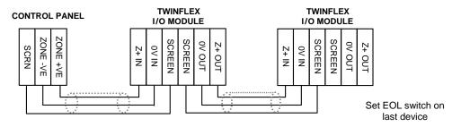
The Twinflex I/O Module can be mixed on the same zone as other types of Twinflex device (eg. Twinflex Multipoint Detectors). The above diagram shows how to make the zone positive, zone negative and screen connections between the control panel and Twinflex I/O Modules. Refer to the instruction leaflets supplied with other Twinflex devices for their equivalent wiring/terminal labelling details.
