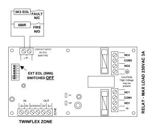
Input with Fault Monitoring
