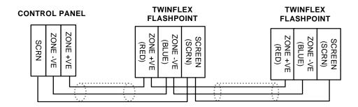
Twinflex Flashpoints can be mixed on the same zone as other types of Twinflex device (eg. Twinflex Multipoint Detectors). The above diagram shows how to make the zone positive, zone negative and screen connections between the control panel and Twinflex Flashpoints. Refer to the instruction leaflets supplied with other Twinflex devices for their equivalent wiring/terminal labelling details.
