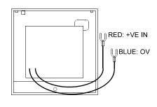
Care should be taken when terminating devices to ensure all cables are correctly sleeved and connections are secure. Improper connections will prevent a system from responding properly in the event of a fire. Please remember that all high voltage testing must be carried out before the installation of the Flashpoint front unit as this may cause damage. It is important to maintain the screen continuity in order to protect against data corruption from interference.
