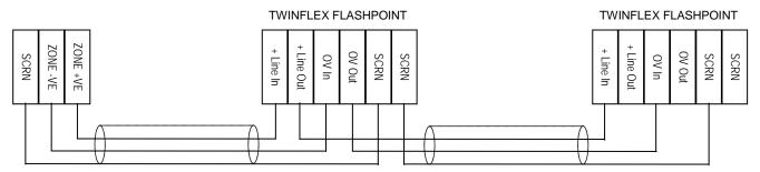
Twinflex Flashpoints can be mixed on the same zone as other types of Twinflex device (eg. Twinflex Multipoint Detectors). The above diagram shows how to make the zone positive, zone negative and screen connections between the control panel and Twinflex Flashpoints. Refer to the instruction leaflets supplied with other Twinflex devices for their equivalent wiring/terminal labelling details.
