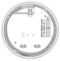
The Loop +ve (positive) IN and the Loop +ve (positive) OUT connections are split within the module. For cable continuity readings at the commissioning stage they must be temporarily removed and connected through. Please remember that all high voltage testing must be carried out before the installation of the electronics, otherwise the electronics will be damaged. Please also note that the SCRN terminal should only be connected to the loop screen and NOT the building earth.
