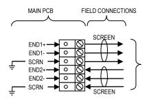
Each loop 1-4 addressable circuits must be connected to its appropriate End 1 and End 2 terminals.
