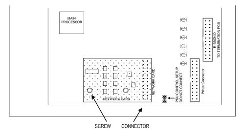
Before any networking facilities may be used, the optional Quadnet network card must be fitted to the control panel main PCB (CIE) as shown above.
