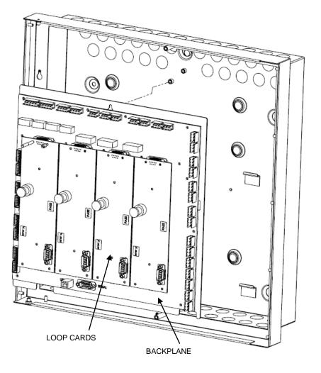
The panel is normally supplied disassembled to make first fix easier. If the panel is already assembled it must be disassembled in order to fix the backbox to the wall.
