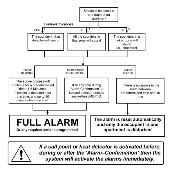
This function affects the smoke detector only, and operates before the control panel enters the Fire state. Thus, the system 'Cause & Effect' does not need to be adjusted, as **Alarm Confirmation takes place before the programmed Cause & Effect sequence is reached**.
