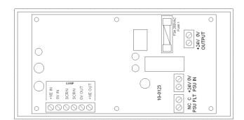
Before installing the module remember to note the serial number of the device (located on the rear of the unit) on to your drawings or configuration sheets to enable you to prove its location later. The address allocation for the device is carried out automatically by the control panel whilst in initialisation mode, so addresses do not need to be set manually. See system installation and operating instructions 26-0353-21, 26-0809-13 & 26-0582-14 for further details.
