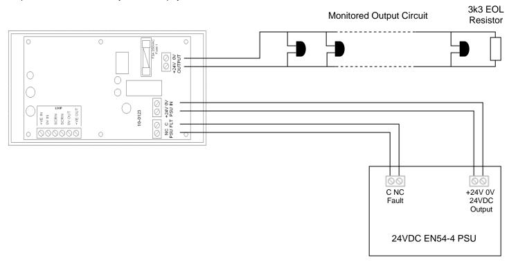
Notes: This module monitors the output circuit only in the quiescent state using a reverse voltage. Any devices connected to the monitored output circuit MUST be polarised and protected from operation if voltage is applied in the reverse polarity. This can normally be achieved by the addition of blocking diodes.
